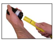
8 Stab pipe completely into fitting so that the mark on the pipe is within 1/8" from the fitting entrance.
