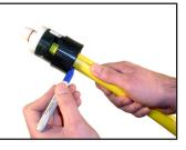
6 If using ID chamfer tool with gauge, check for proper chamfer by inserting pipe on gauge up to the o ring. With proper chamfer, o ring will begin to enter pipe.
